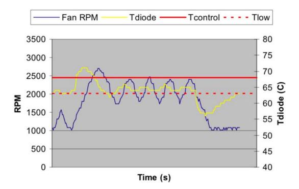
An alternate would be to consider a slightly larger value such as  $T_{RANGE} = 10$  °C. In this case the design is trading off the acoustic margin for thermal margin.
